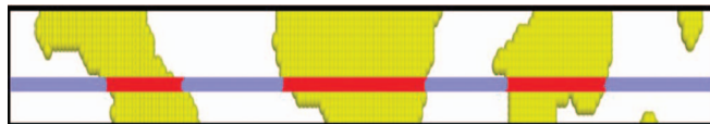
FIG. 8. Chords are defined by the intersection of straight lines with the interfaces in the phase separating system. In this bidimensional example, the red segments belong to the dense phase (yellow areas) and their length give the chord length of the dense phase.
